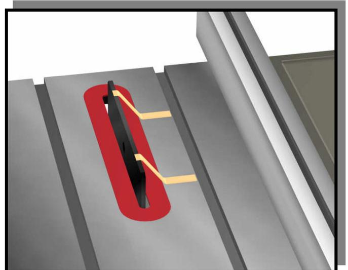
To keep the **MasterPlate** positioned correctly and prevent it from rotating on the arbor shaft, tape the ends or edges as shown. This will keep the **MasterPlate** stable while you are measuring/setting with your **MasterGage/Classic**.
