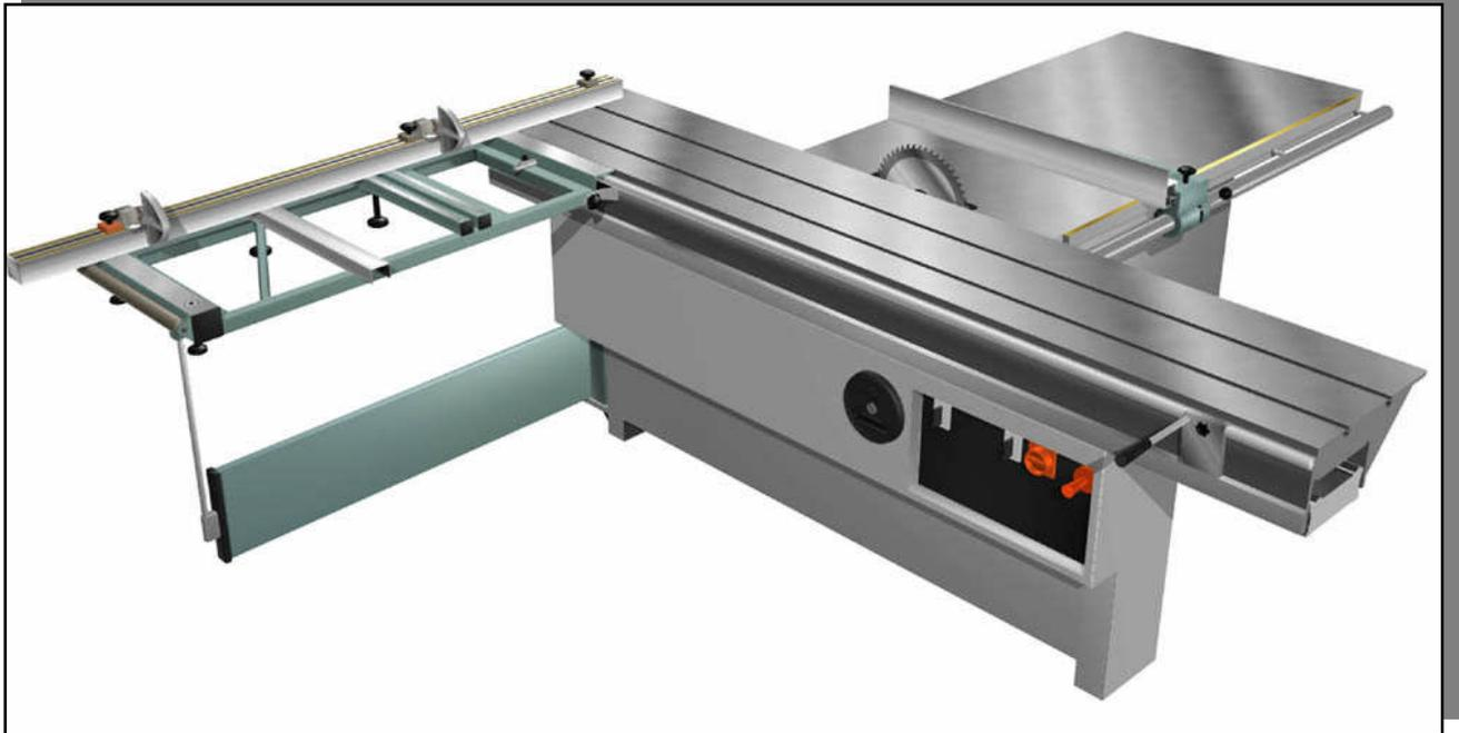
A little background on sliding table saws. They were originally developed by European saw manufacturers for the 32 mm system for construction of cabinets and case goods. The 32 mm system requires precision machining of sheet goods such as MDF (medium density fiberboard) and melamine for the fabrication of case goods.
