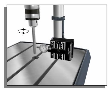
Check spindle run out by rotating the check by hand and reading the dial indicator at the tip if the Precision Rod
