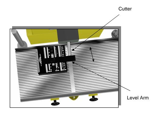
Set the cutter depth required and lock table stops.
