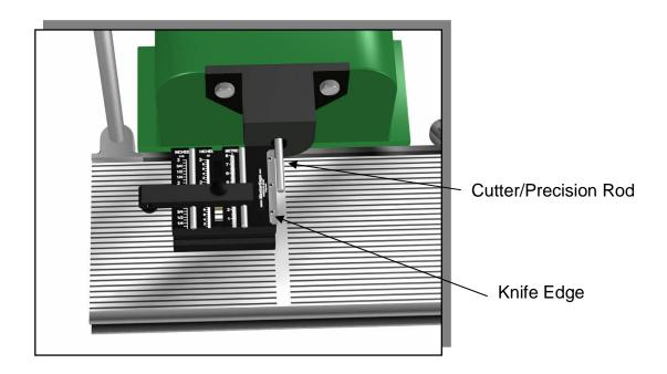
Use the ½ inch by 4 inch Precision Rod for alignment. The Precision Rod with it's straight, smooth surface is far more accurate than using a cutter for alignment.
