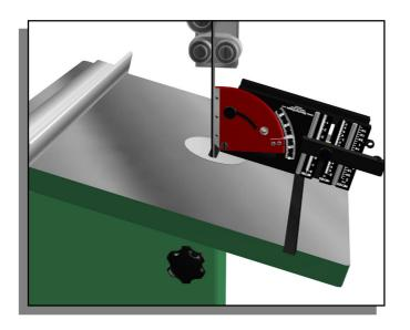
Set any angle desired from 0° to 45°, to an accuracy of 0°, 15 minutes [1/4 degree]. Also, verify any existing table tilt angle.
