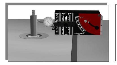
Checking spindle run out by rotating spindle by hand.
